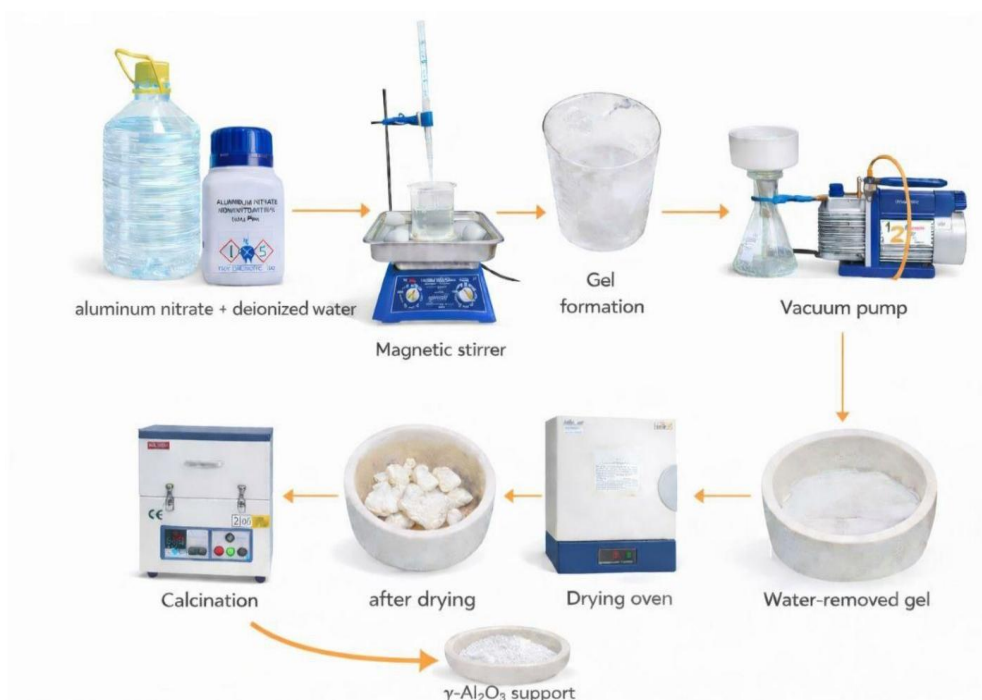
Figure 1. Manufacturing steps of \gamma -Al 2 O 3 support
