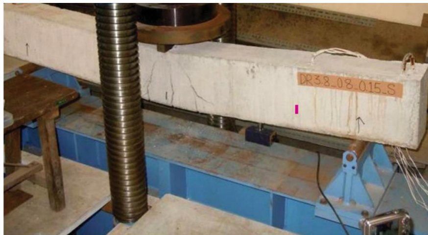
Figure 3. Failure modes: DR3.8_0.8_0.15 [Satadru et al., 2015].
