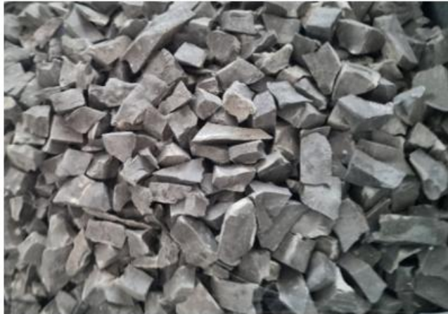
Figure 1. Artificial aggregates made from a mixture of fly ash and epoxy resin
