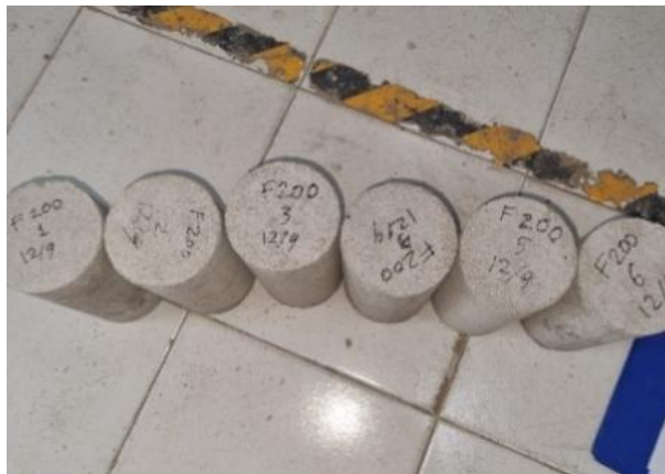
Figure 4. Foamed concrete specimens after 28 days of curing
