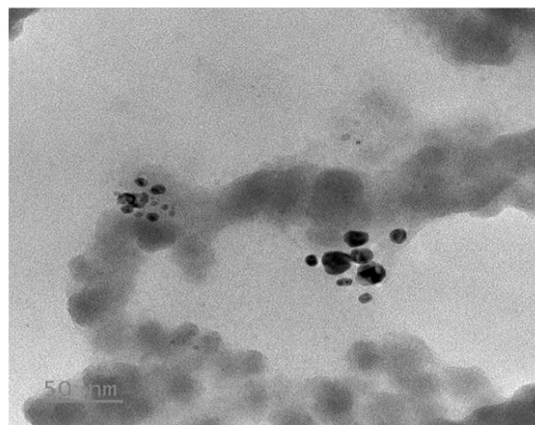
Figure 3 TEM images of the CQD1 (a), CQD2 (b), and CQD3 (c) samples, fabricated at hydrothermal temperatures of 170°C, 200°C, and 230°C, respectively.
