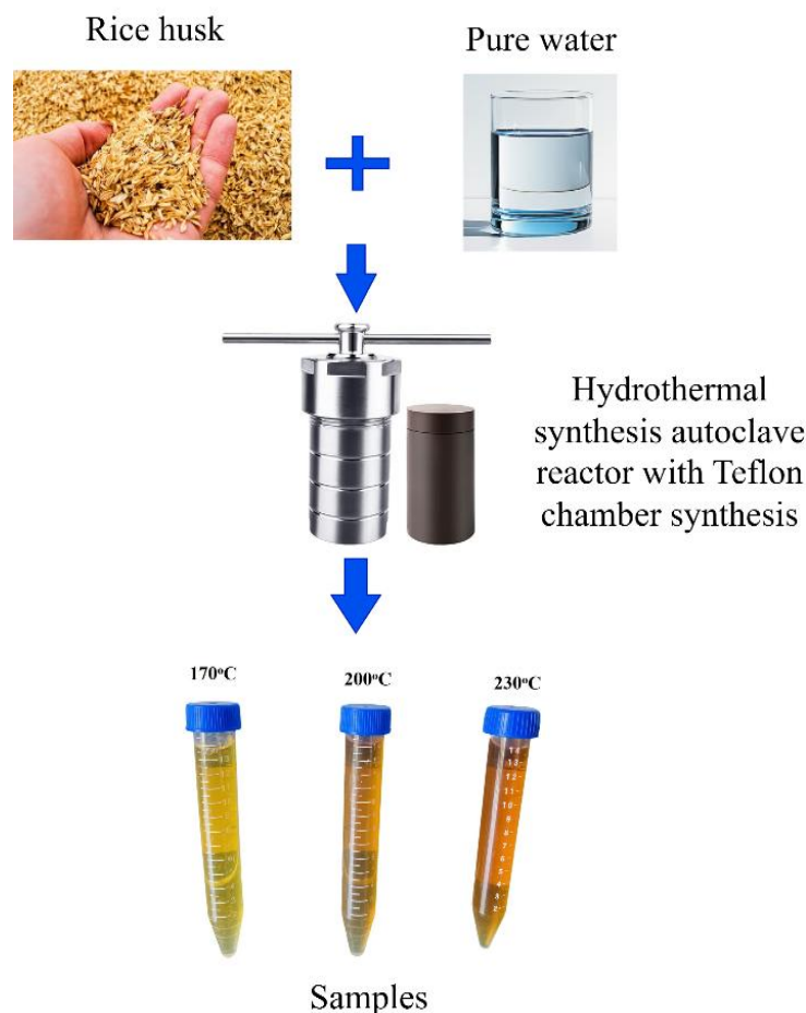
Figure 1 The fabrication procedure of Carbon quantum dots
