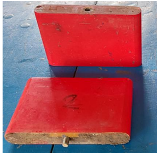
Figure 2 Variation of rectangular porous baffle block angle (a) Angle 180; (b) Angle 300
