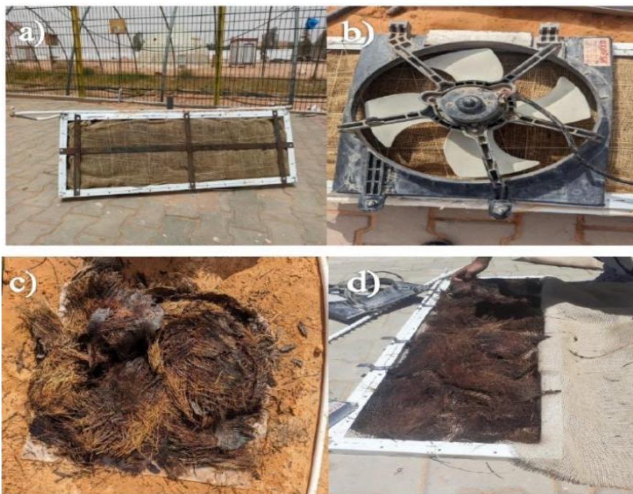
Figure 5 Components of Fan-Pad cooling system: a) Evaporative cooling pad, b) Fan, Palm leaf, c) Palm leaf, d) Arranging palm leaf inside an evaporative cooling pad
