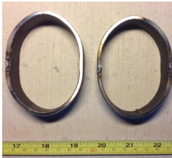
Figure 10 Test Specimen with welded seam oriented at 0 degrees (left) and 90 degrees showing limited effect of seam placement on deformation.
