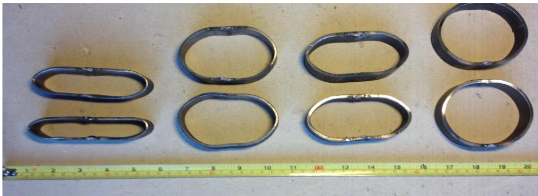
Figure 4 Complete deformation of 75 mm Test specimen, series increasing wall thickness from left to right, for 0.250 kJ potential energy dissipation, showing good repeatability of experiment
