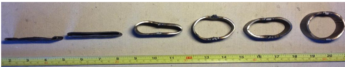
Figure 5 Complete Deformation of 50mm series test specimen for, increasing wall thickness from left to right, 0.25 kJ potential energy dissipation.
