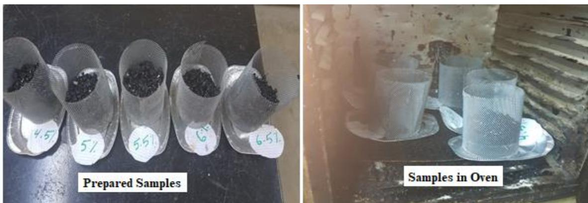
**Figure 4.** Drain down test
