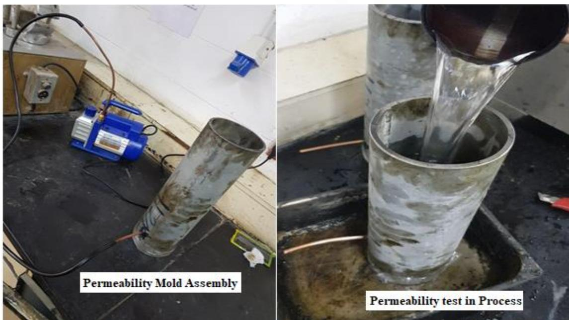
Figure 7. Permeability test of Porous Asphalt Concrete
