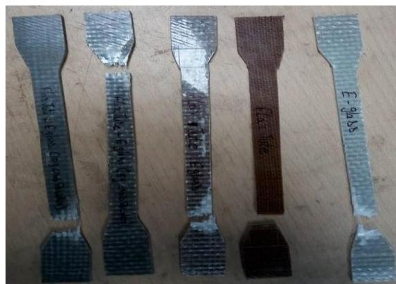
**Figure 13)** the specimens after tensile test
