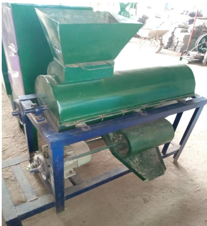
Figure 1 Pictorial View of the Maize Shelling Machine
