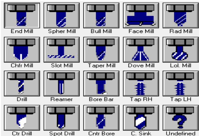
Figure 6 Schematics of Various Types of Cutting Tools
