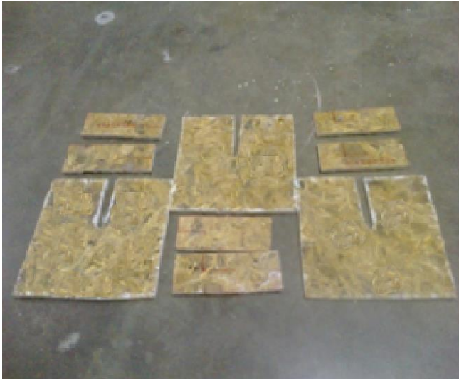
Figure 1 Banana/Glassfibre hybrid composite specimens as per ASTM standards
