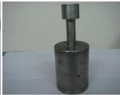
Figure 7 Assembly of compression. (Bottom plate, Punch and (Bottom plate, Punch and body)
