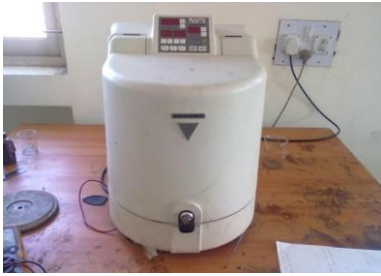
Figure 1 Ball milling setup
