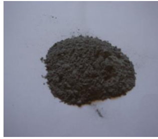
Figure 2 After ball milling (or) mixture of pure aluminium
