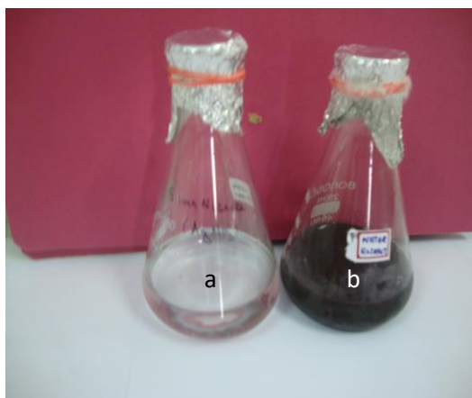
Figure 2 (a) 1mM silver nitrate solution, (b) 5ml of leaf extract in 100ml of 1mM silver nitrate after 48hrs of incubation
