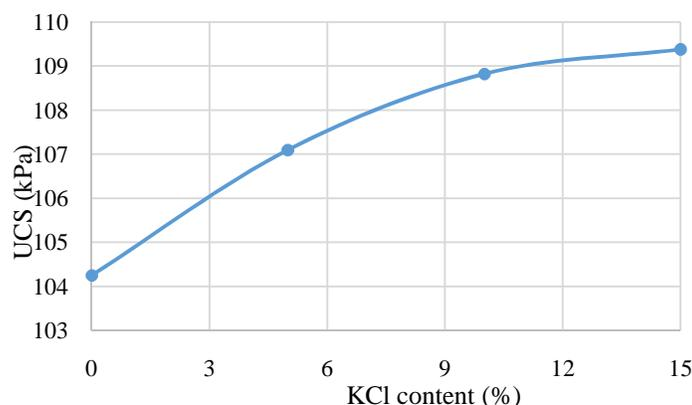
**Figure 3** Effect of potassium chloride on UCS
