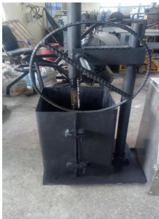
Fig 2: Fabricated mechanical waste compactor.
