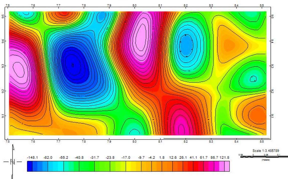
**Figure 5** The first vertical derivative aeromagnetic map of the study area (nT)
