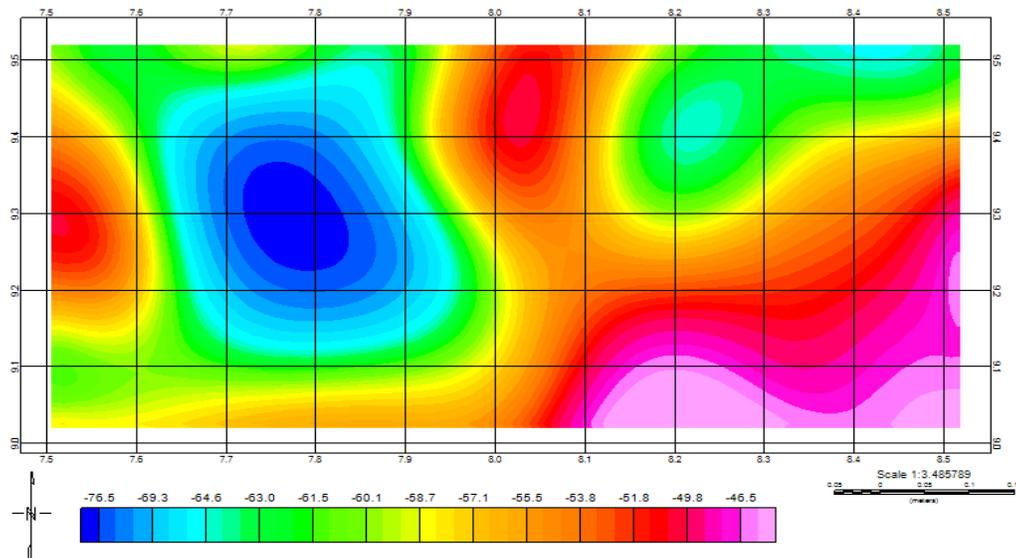
**Figure 2** Total aeromagnetic intensity composite map of the study area (nT)
