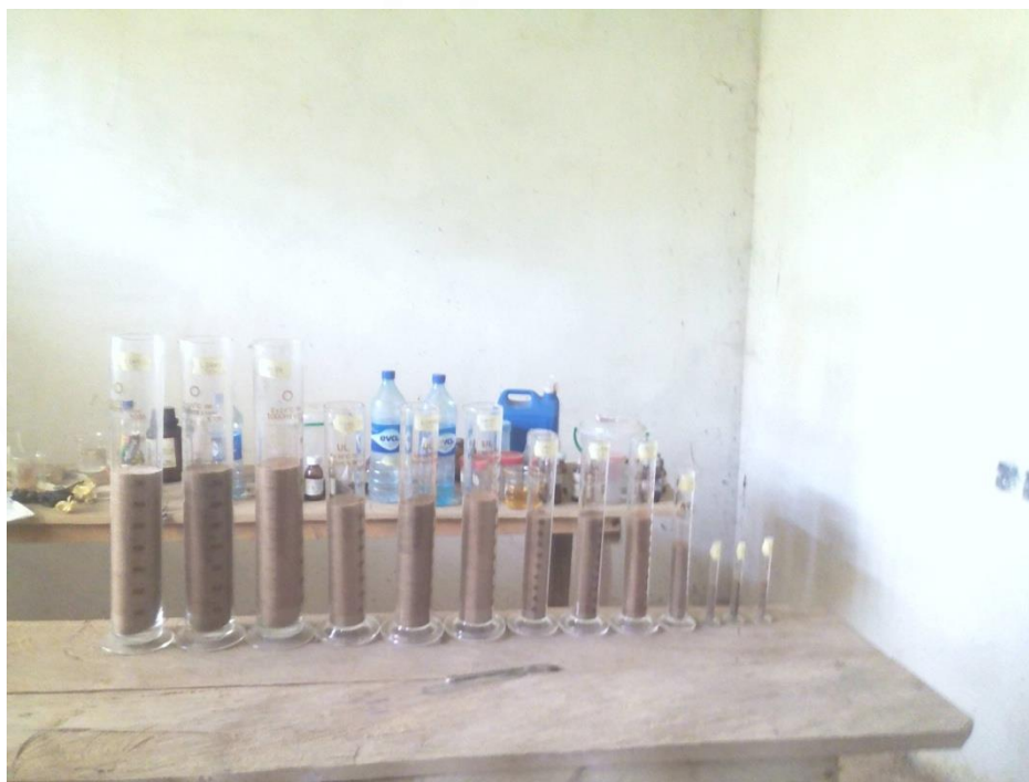
Figure 1 Experimental set-up for capillarity diffusion of Crude Oil in Soil Environment
