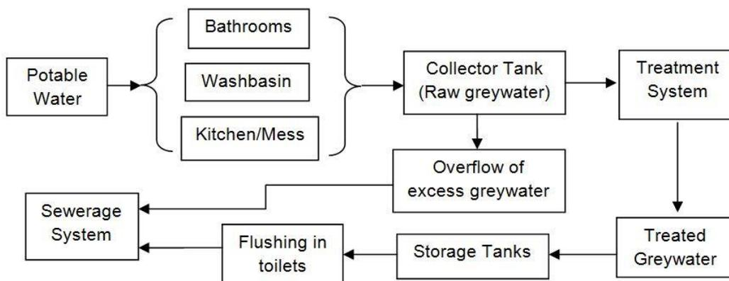
**Figure 2** Flowchart of the various components involved in the greywater treatment system
