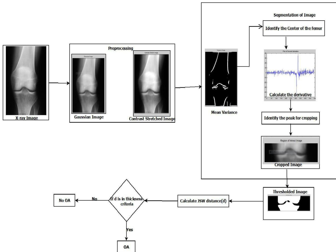
**Fig.5.** Automated System Design Architecture
