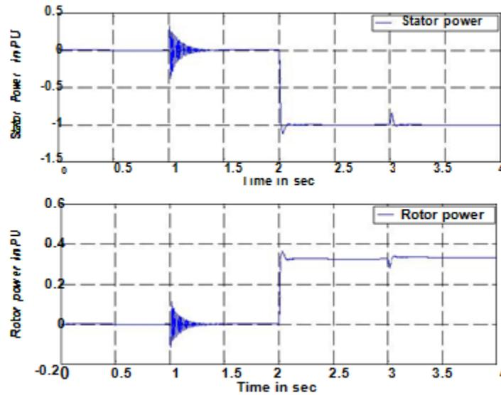
The stator active and reactive power is controlled at the instant of 2 and 3 sec as
