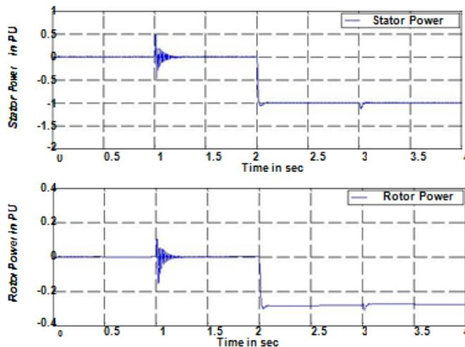
So in the graphs we can see that stator and rotor is supplying power to the grid in super-synchronous mode after 2 sec, here negative value means generating the power and positive value means absorbing the power from grid.
