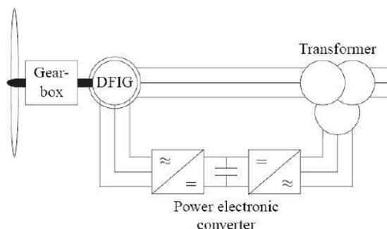
**Figure 1** Wind turbine with a doubly-fed induction generator (DFIG)
