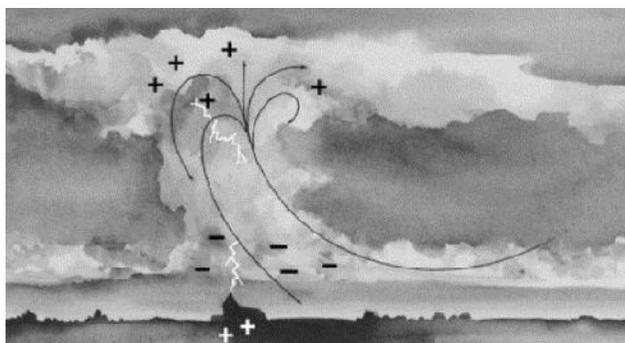
**Figure 2** This is a typical cloud and its polarization: the lower part of a typical cloud has a negative charge and the upper part has a positive charge [2,6]
