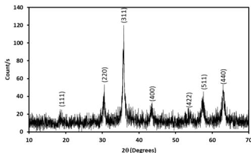
**Figure 1** The XRD patterns for the prepared  $\text{Fe}_3\text{O}_4$  nanoparticles.
