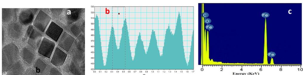
**Figure 2** (a) TEM image, (b) Interplanar distance distribution histogram and (c) The EDS spectra of the  $\text{Fe}_3\text{O}_4$  nanocubes.
