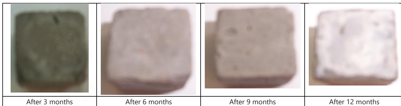
Fig. 5 -The OPC cement pastes incorporated SDA (PS5) and immersed in 4 % MgSO_4 up to 12 months.
