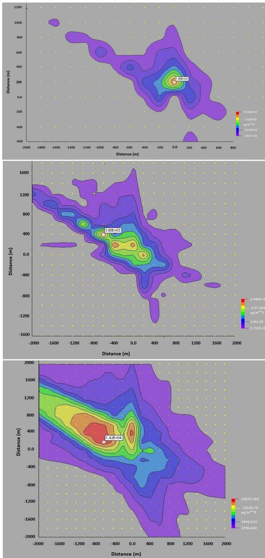
Figure 4: Effect of number of sources on the affected area for hourly CO<sub>2</sub> concentration with stack height of 4m (upper: single source, middle: ten sources, down: 200 sources)
