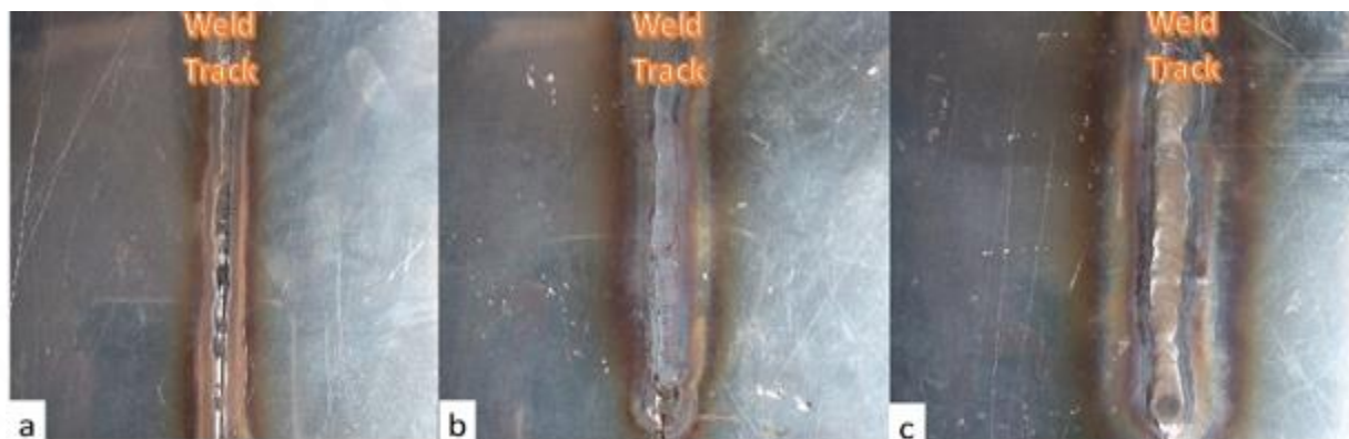
Figure 12 Topographies of the welds under different grain welding conditions: (a) 10A (b) 30A (c) optimized condition
