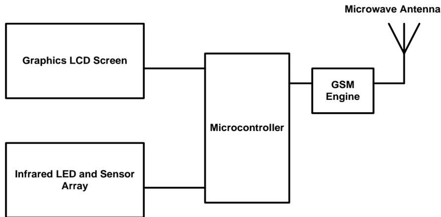
**Figure 1:** Block diagram of the touchless phone
