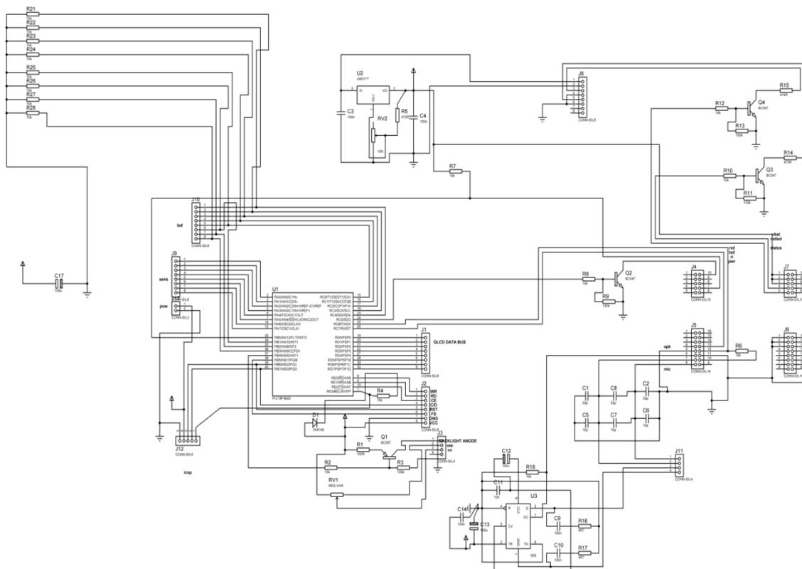
**Figure 2:** A schematic-circuit representation of the touchless phone
