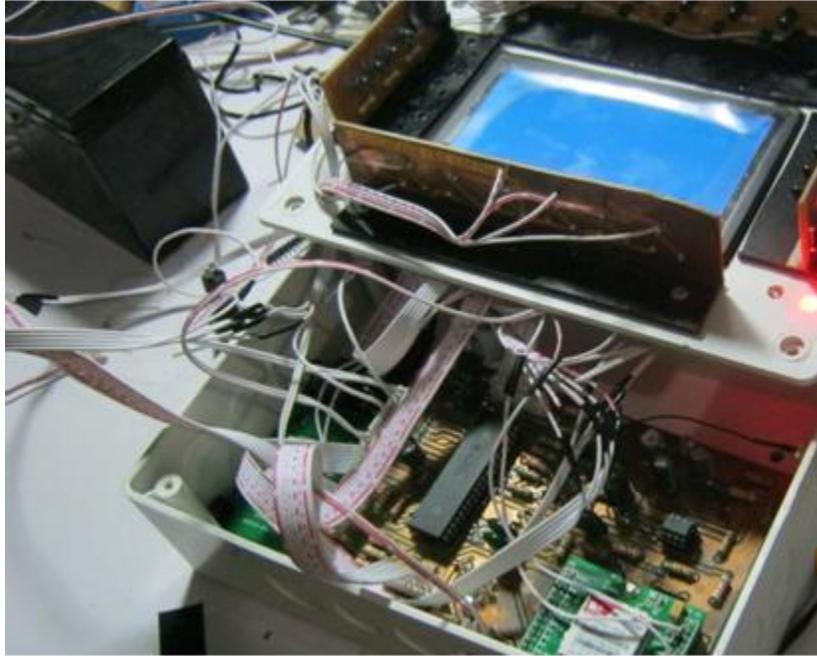
**Figure 8:** Mounting the circuit to the casing
