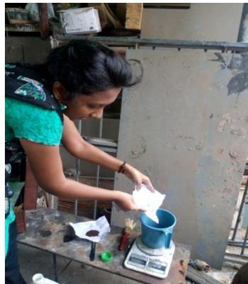
**Figure 3** Mixing of copper powder in resin
