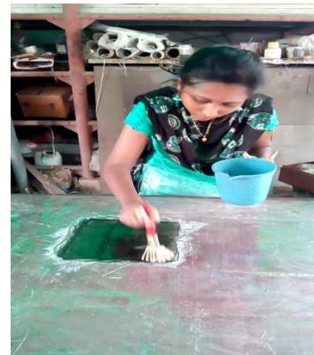
**Figure 4** Applying of filler material on the fibre mat
