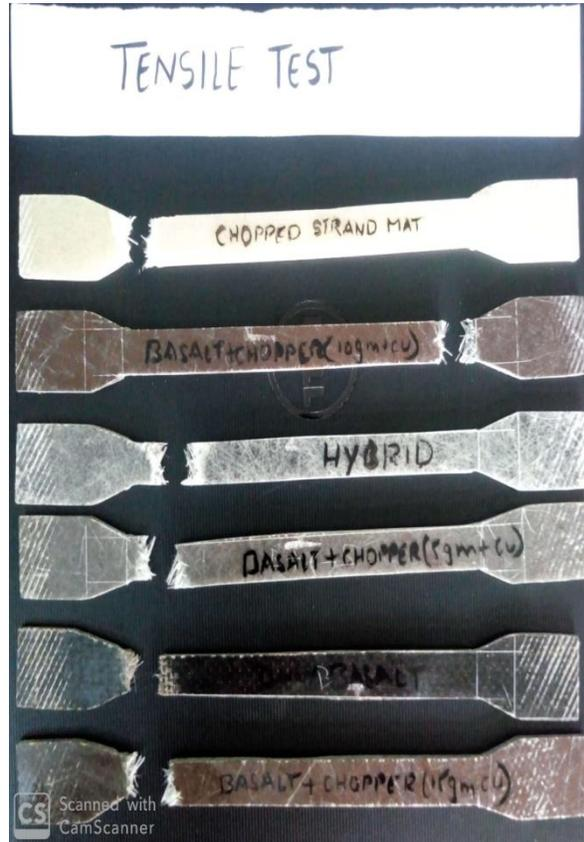
**Figure7** Specimens after failure
