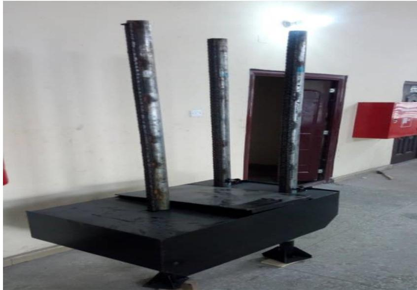
**Figure 6** Fabricated Jack-Up Structure
