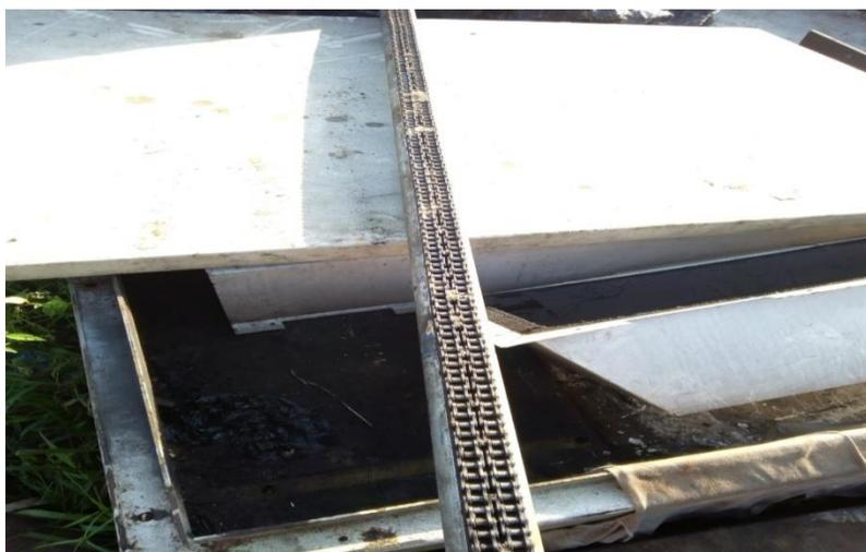
**Figure 2** Duplex Chain Leg Design
