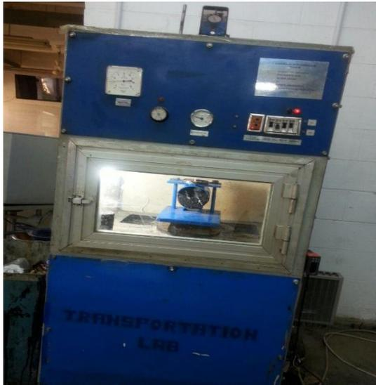
Figure 8 PRLS and the cyclic shear stress test
