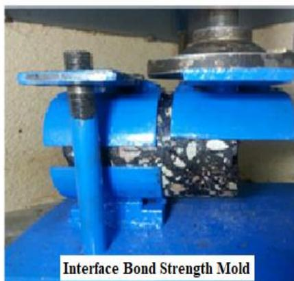
**Figure 6** Interface Bond Shear Strength Mold
