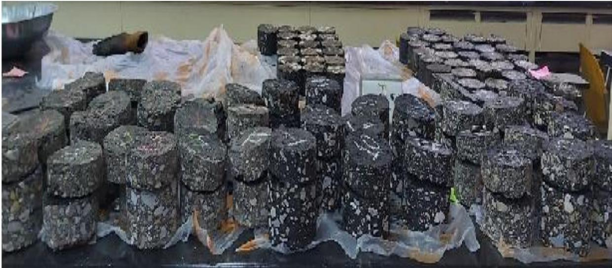
**Figure 5** Part of the Core Specimens Obtained
