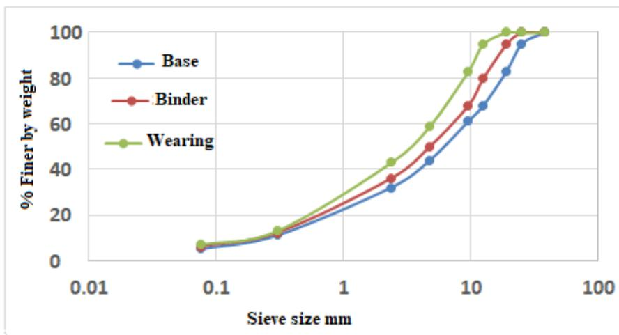
**Figure 2** the Aggregate Gradation According to SCRB, 2003
