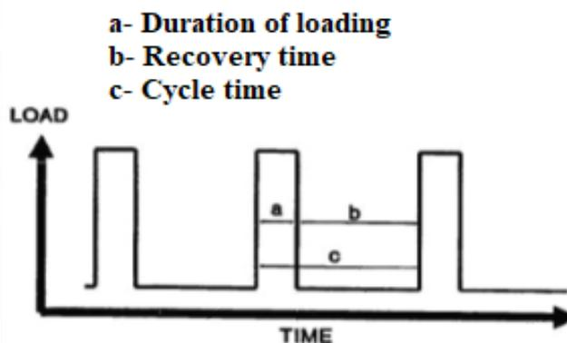
**Figure 7** Cyclic Shear stress loading sequence
