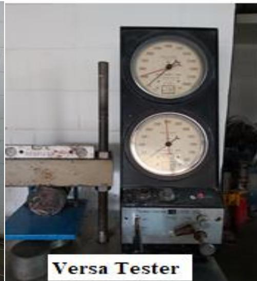
Figure 9 Interface Bond Shear Strength Testing
