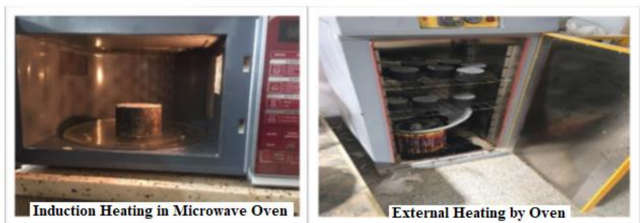
Figure 6 Heating techniques adopted
