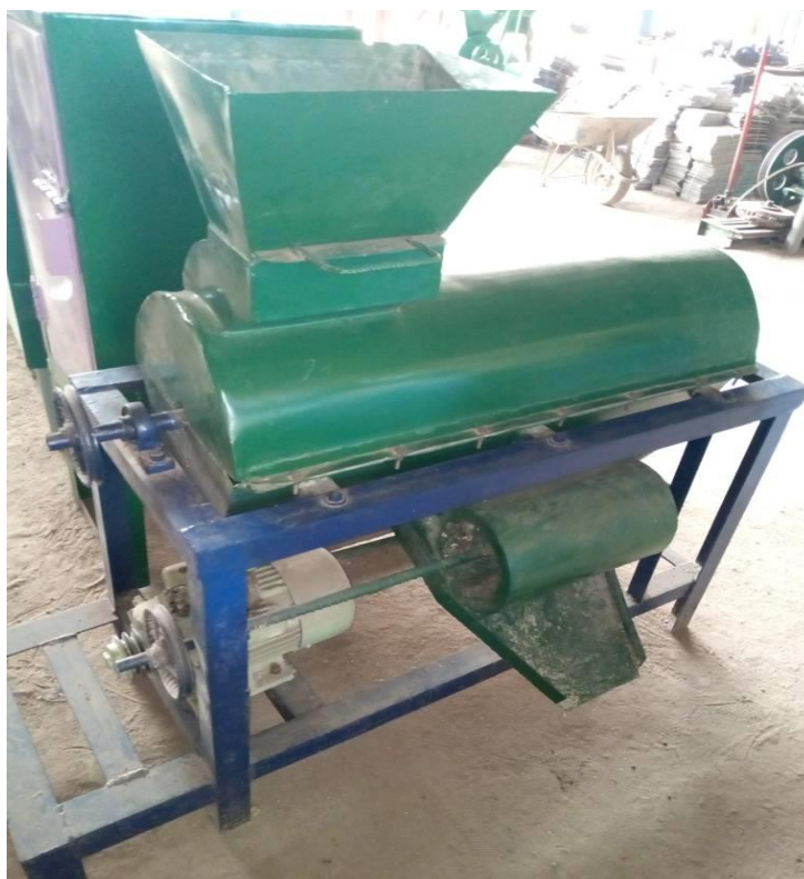
Figure 1 Pictorial View of the Maize Shelling Machine
