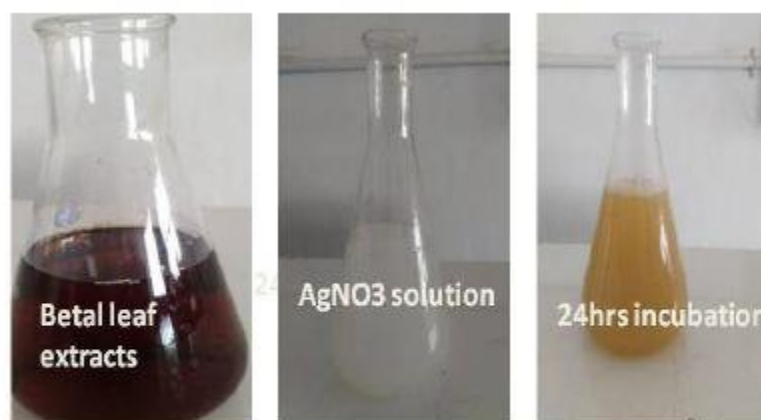
Fig 3: Colour change of betel leaf extracts containing AgNPs before and after synthesis.
