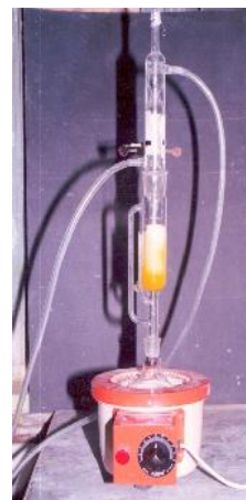
Figure 1 Soxhlet Extractor for extraction process of Curcuma longa
