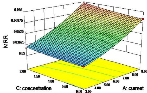
**Figure 5** Effect of Current and Concentration on MRR at pulse on time 150 $\mu$ s
