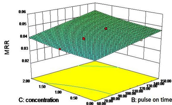
**Figure 4** Effect of Concentration and Pulse on Time on MRR (current 6 amperes)
