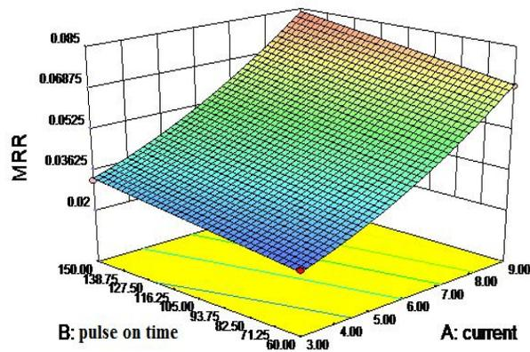
**Figure 3** Effect of  $T_{on}$  and current on MRR at concentration of 2 g/ltr.
