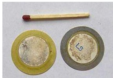
Figure 4 Metal Disks with Piezo Material, Used in Buzzers or as Contact Microphones (Zarnik et al., 2009)
