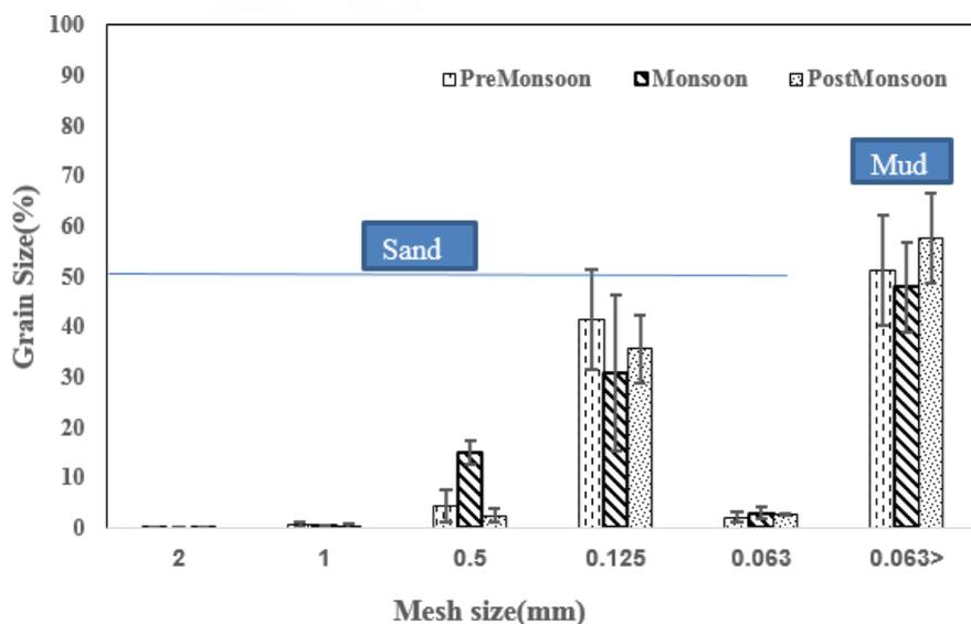
**Figure 2** Average percentage in grain sizing (Mean±SD) in different seasons by sieve size (mm).
