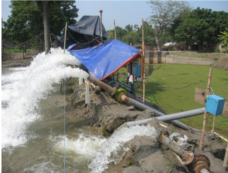
Photograph 1: Draining out of congested water from a sluice gate of a polder in order to cultivate Boro rice in Tala upazila of Satkhira district. Photo Credit: Author.
